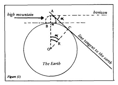
The horizon should be drawn on top of the mountain (But how?) Abu Raihan then by using an instrument similar to today's telescope overlooked the surface of the earth and measured the angle ( $\ll$ ) between the horizon
